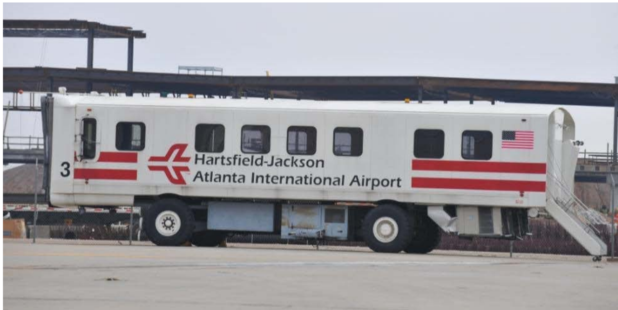
There are three PlaneMate vehicles with an 85-passenger capacity.
