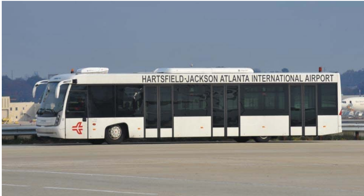
There are four COBUS 3000 vehicles with a 75-passenger capacity.
