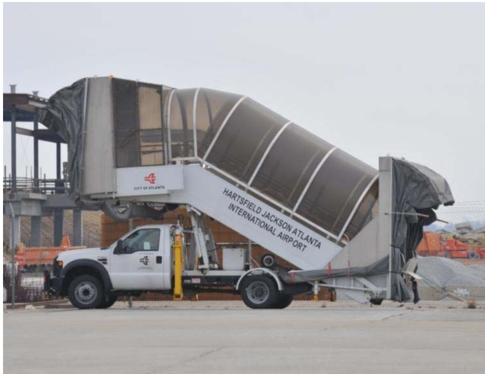
There are two vehicle-mounted passenger stairs capable of accommodating aircraft ranging from the B737/MD-88 to the B747-400.
