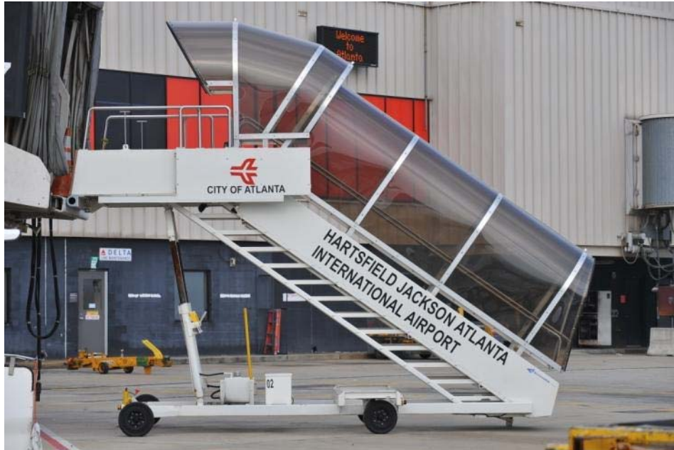
There are two towable passenger stairs capable of accommodating aircraft ranging from the E170 to the B737/MD-88.
