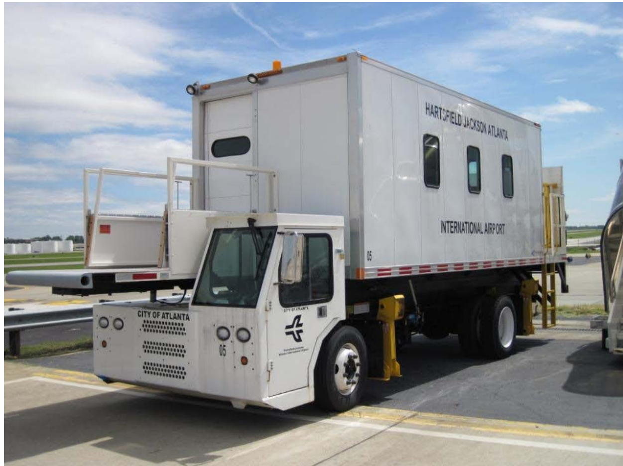
The ambulatory lift is capable of accommodating aircraft ranging from the E170 to the B747-400.
