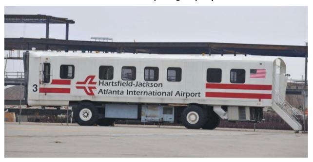
There are two PlaneMate vehicles with an 85-passenger capacity.
