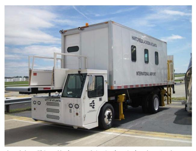
The ambulatory lift is capable of accommodating aircraft ranging from the E170 to the B747-400.
