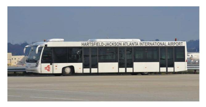
There are four COBUS 3000 vehicles with a 75-passenger capacity.
