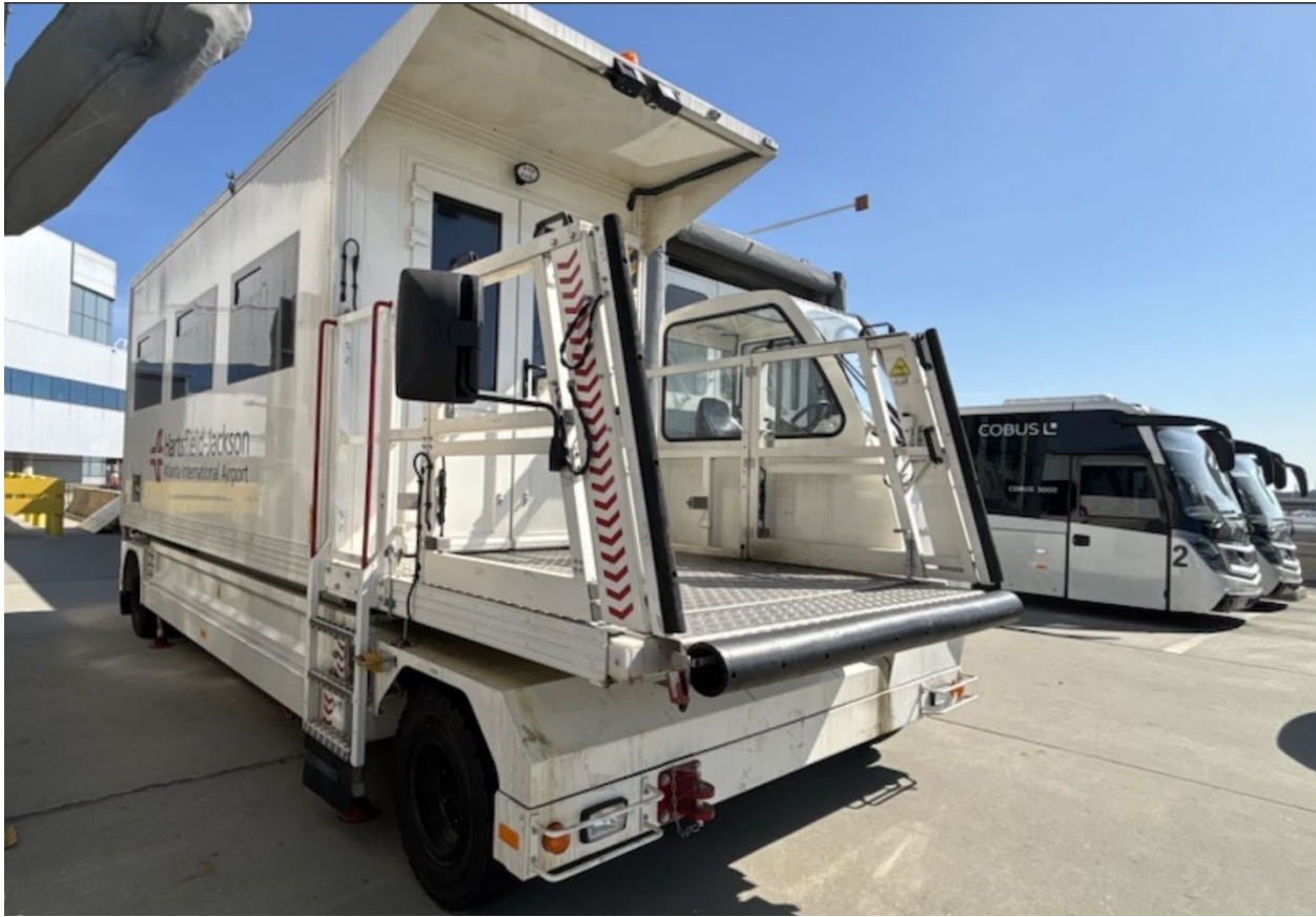
The Mallaghan ML6100D ADA ambulatory lift is capable of accommodating aircraft ranging from the E170 to the B747-400.
